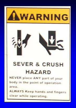
Sheet metal tools exert powerful force to bend and cut material, and present severe dangers of crushing and severing extremities. Pay attention to all posted warnings and keep hands away from the working area.
