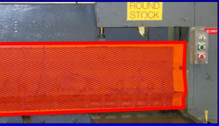
The shear guard should be set as low as possible, allowing only enough room for sheet stock. Its purpose is to keep your hands away from the point of operation, and must NEVER be removed.
