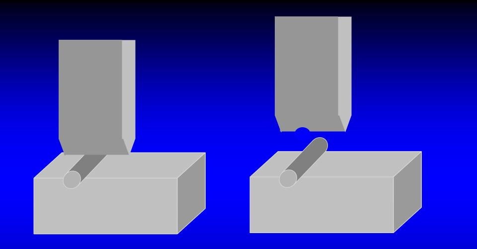
Cutting material other than sheet metal stock can damage the shear blade, creating an unsafe tool for the next person to use the machine.
