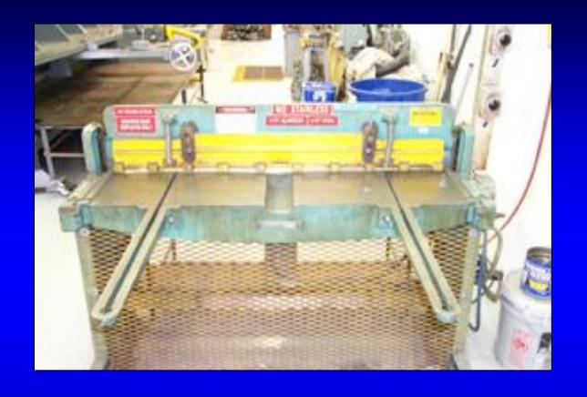
A shear is a tool used to cut straight edges into sheet metal stock.
