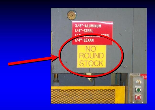
Remember that the shear is for sheet metal only.
