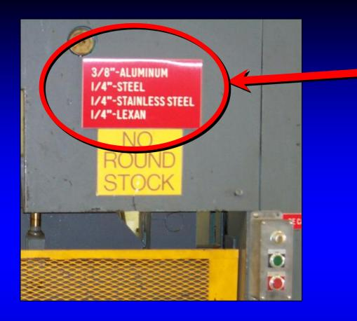
Before cutting sheet metal with a shear, ensure that it is rated to cut the gauge of sheet metal you're working with. The gauge rating is generally marked on the machine.
